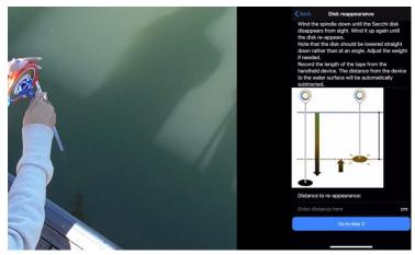
Wind it up again until the disk reappears. The disk should be lowered straight down, not at an angle. Record the length of the tape.
